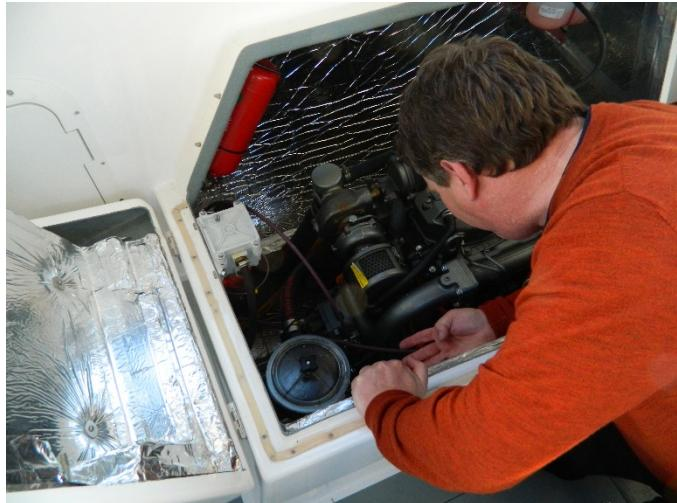
the coolant so that you can see the level at a glance. It's worth taking the cap off the heat exchanger to check there's actually coolant in the engine, a blockage in the expansion pipe can leave plenty in the bottle but none where it's needed.
